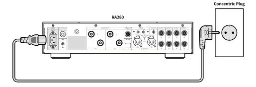
⚠ Caution : When disconnecting the power cord, always disconnect the power outlet first with the power switch off.
